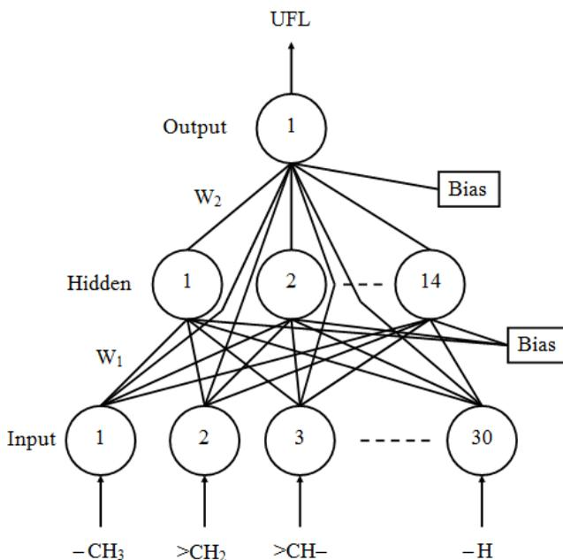
Figure 1: Schematic representation of the 30-14-1ANN used to predict the UFL of pure compounds from their structure groups
